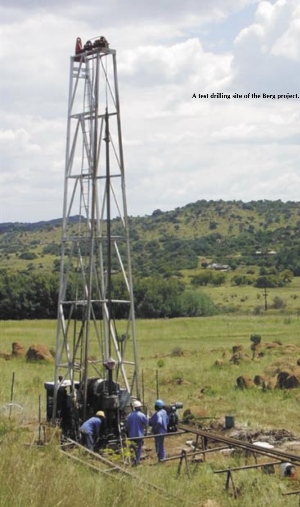
Drilling of borehole BD6 which successfully intersected UG2 Reef.
